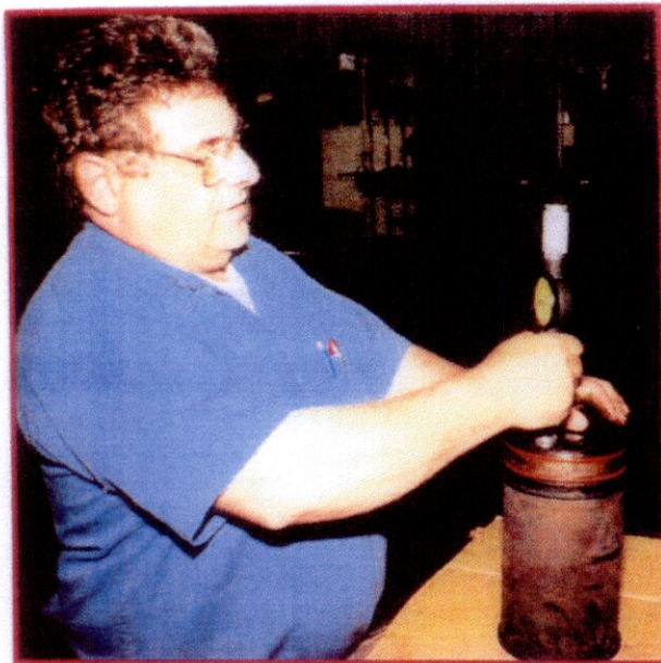
Evans' diesel fleet rep Al Improta uses a dial bore gauge to measure cylinder taper on cylinder liners removed from the Detroit Diesel Series 60 after 500,000 miles. "Every cylinder was within original OEM specifications," he observes.
